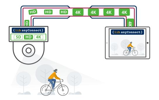
AnyConnect Adaptive Bitrate Streaming encodes video from a connected camera with multiple and variable bitrates in HD base and 4K UHD enhancement layers. Mobile apps adapt video quality based on their available network and CPU capacity.
